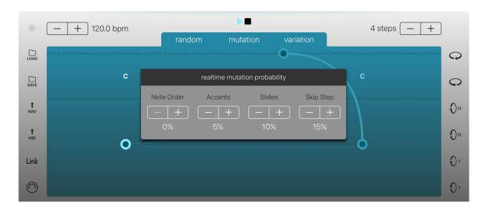
The realtime mutation engine takes your pattern and introduces semi-predictable variations during playback. Four different parameters can be individually processed using the engine.
